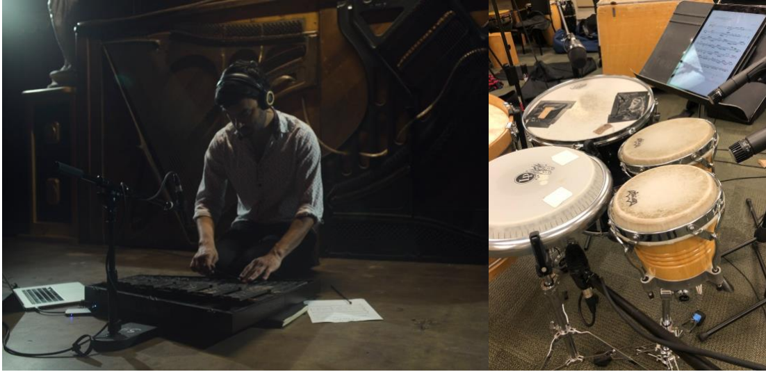
Figure 2. Examples of microphone choice in the EIP. James Parker's "Baptism of Wind and Waves" (left) is best treated with a small diaphragm condenser microphone to capture the shimmer of the bells. Caleb Evans' "Conversation" (right) features exclusively drums and is best recorded with dynamic microphones.
